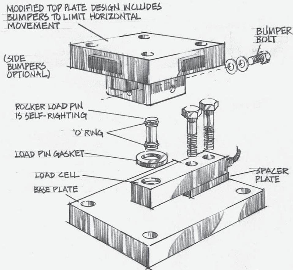
*Mettler Toledo's self-aligning weigh modules accommodate high horizontal forces.*
