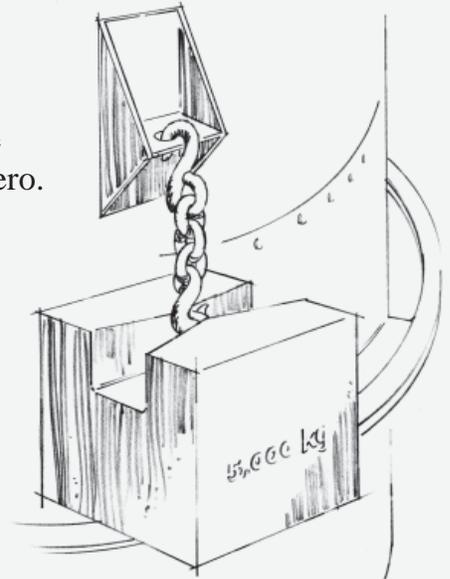
*Hanging test weights will also require a hoist or forklift to place the weights.*
