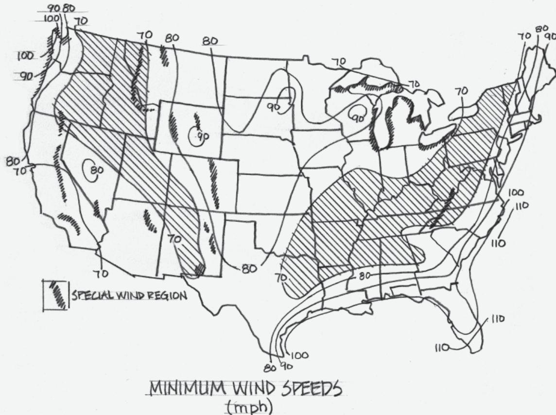
Wind load calculations need to be run for full and empty tanks using an acceptable figure for maximum wind speed. Check local codes for guidelines.
