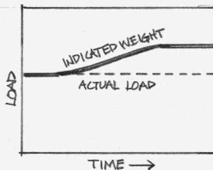
With your tank scale built and ready to put into service, the only task that remains is calibration and verification. Calibration is simply instructing the system when to indicate zero (really the tare, i.e., the weight of the empty tank) and when to indicate the maximum weight, i.e., when the tank is full. Verification documents the actual performance of the scale from zero to maximum and from maximum to zero.
